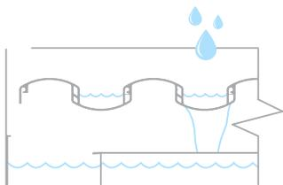
The unique louver profile allows the louvers to interlock, creating the largest rain channels in the industry. Thus, allowing for more water to flow freely into our 360 degree integrated gutter system. StruXure's patented Pass Through Gutter technology allows for rain water to pass from one independent zone to the next allowing for superior drainage performance.
